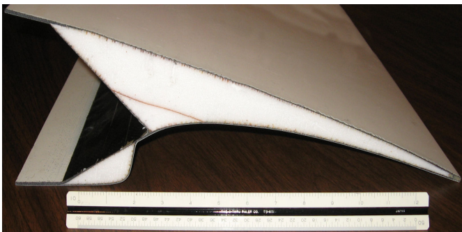
Photo 2 This executive jet flap is manufactured with GRP skins and multiple foam cores with internal bond lines making this part extremely difficult to inspect using traditional NDT technologies.
