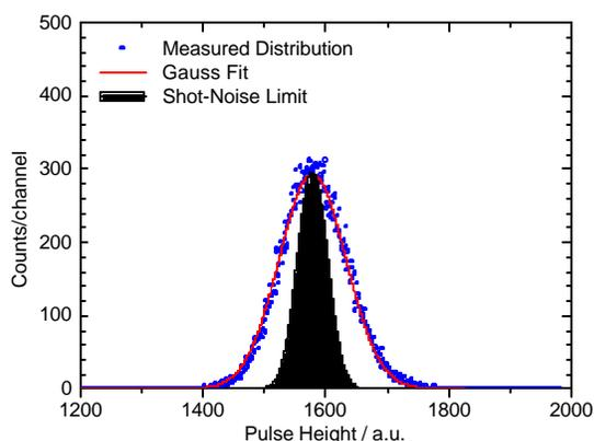
**Figure 3:** Pulse height distribution of recorded single camshaft pulses at 5 keV. The shot-noise contribution is included for comparison.
