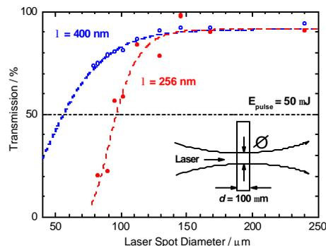
**Figure 2:** Nonlinear absorption losses in neat water ( $d = 0.1 \text{ mm}$ ) as a function laser focus ( $E = 50 \mu\text{J}$ ). Laser wavelengths are as indicated.
