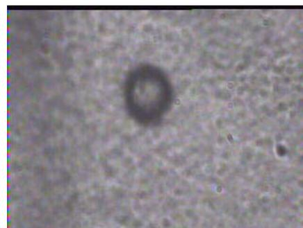
**Figure 2 .** Preliminary Image of UV 'ring', reduced by 100x, produced in homogeneous Gafchromic film – the outer ring is 10 $\mu\text{m}$  in diameter and 1.2 $\mu\text{m}$  in width.
