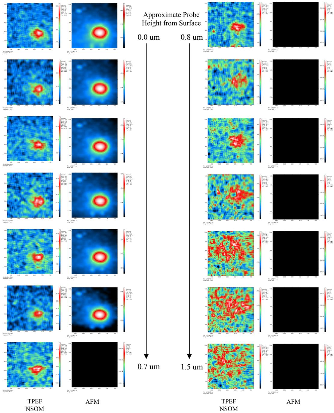
Figure 5. Height Study of RhB Spheres by TPEF NSOM with 820 nm Excitation (Field of view is 3.5  $\mu\text{m}$  x 3.5  $\mu\text{m}$ )
