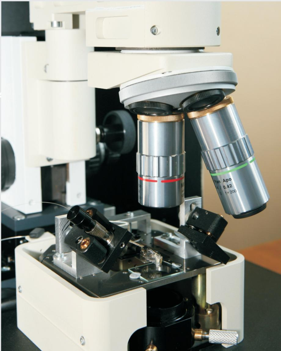
**General view of a Photon Scanning Tunneling Microscope (PSTM) configuration based on the MoScan-F NSOM platform. An evanescent wave is generated at the face of a prism, slide or side polished fiber**
