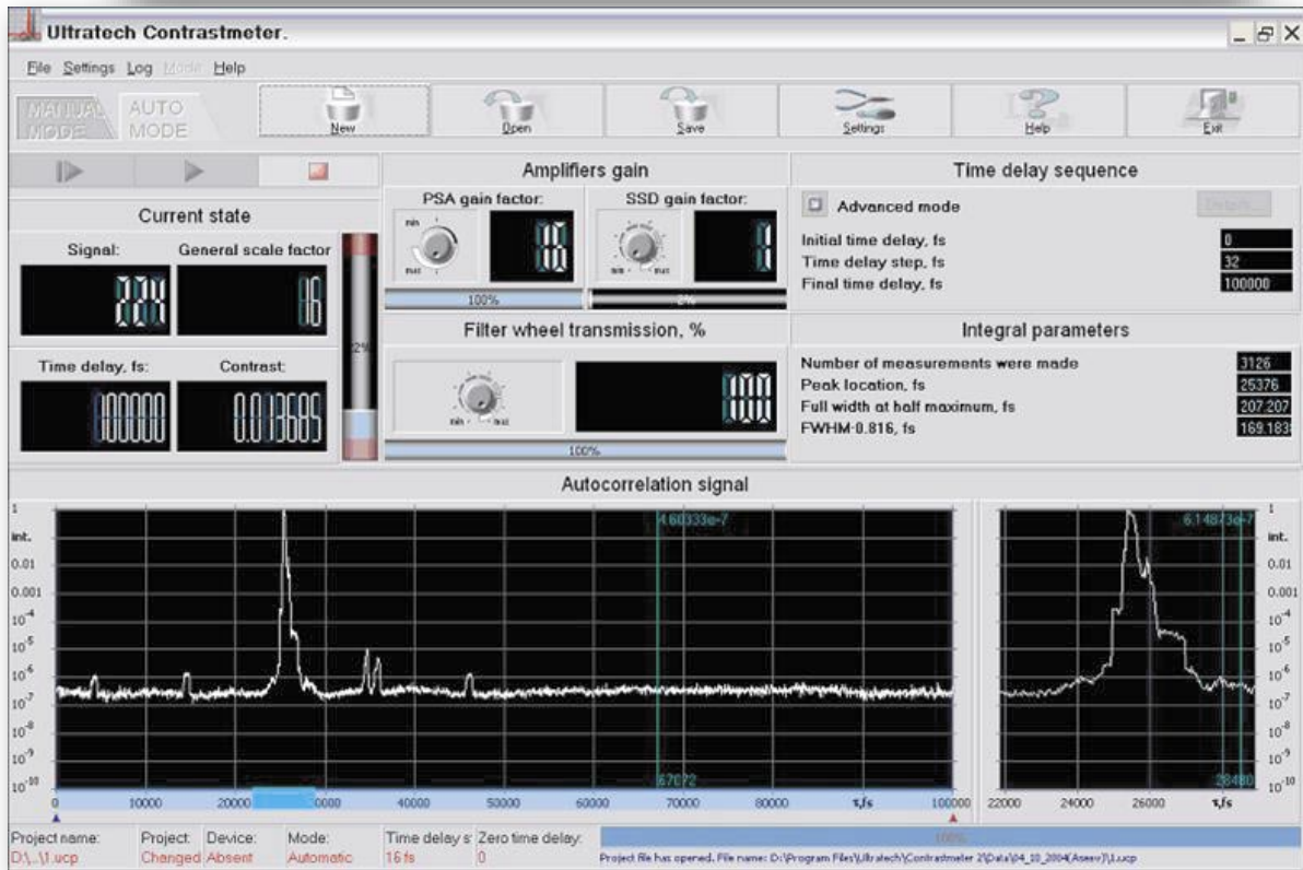
Third order cross-correlation function of laser pulse (Cr:forsterite regenerative amplifier)
