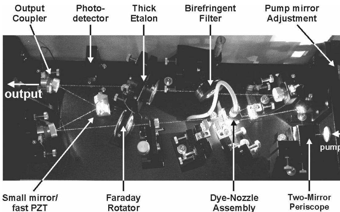
Fig. 3. Top view of combined CW single-frequency ring laser in Dye laser configuration: a picture is given of the laser in operation, real beams of the dye laser and the pumping laser are visible.
