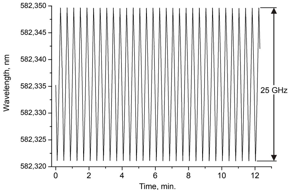
Fig. 7. Automatic smooth scanning of Dye laser frequency in regime of active frequency stabilisation.
