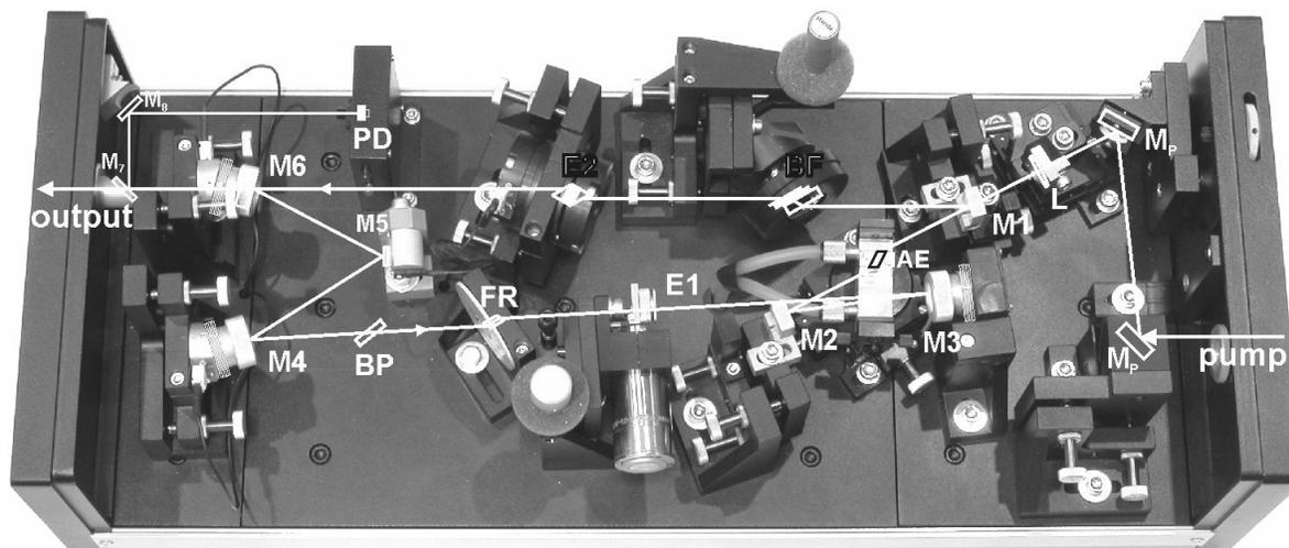
Fig. 2. Layout and top view of combined CW single-frequency ring laser in Ti:Sapphire laser configuration:  $M_p$  - pump mirror, L - lens, M1 & M2 - spherical mirrors, M3, M4, M5 - flat mirrors, M6 - flat output mirror AE - Ti:Sapphire crystal, BF - 3-plate birefringent filter, E1 - thin Fabry-Perot etalon, E2 - thick Fabry-Perot etalon, FR - Faraday rotator, PD - photodetector, M7 & M8 - auxiliary mirrors.
