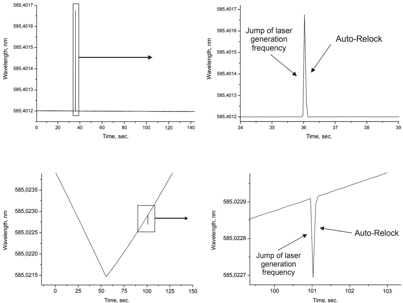
Fig. 8. Demonstration of Auto-relock function work in regime of fixed wavelength and in regime of automatic smooth scanning of Dye laser frequency.
